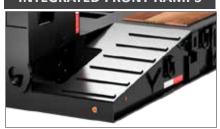
Low profile built-in integrated deck ramps.
