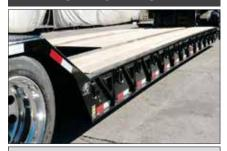
With a standard deck height of 18", Globe Trailers have lower overall height, which allows taller loads to be hauled.
