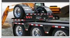
Globe Trailers has a patent on the hydraulic flip axle design. It allows for less down time when operating the flip axle and it can be easily detached when required.
