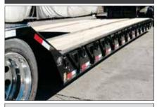
With a standard deck height of 20", Globe Trailers have lower overall height, which allows taller loads to be hauled.
