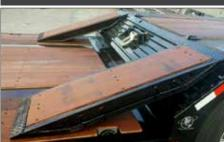
Adjustable sliding transition ramps with wood covering for traction. Ramps are removable.
