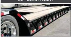
With a standard deck height of 22", Globe Trailers have lower overall height, which allows taller loads to be hauled.
