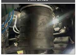
30K pound rated large diameter air bags are standard. This allows for lower operating pressure and higher capacity when needed.
