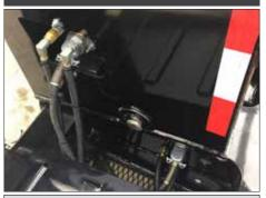
Air, electric and hydraulic (when applicable) fittings are all centrally located at the base of the gooseneck inside a bolster. This makes for quick and easy connect and disconnect. The fittings are protected from possible contact with equipment being loaded or unloaded.
