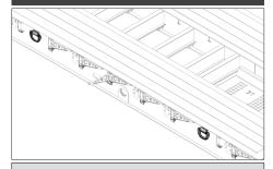
Lift & Tie down rings on both sides of the main deck.
