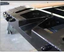
V-Style guide with front tapered beams helps position the gooseneck locking pin, which makes hooking up to a Globe Trailer fast and easy. The locking pin guide rim helps prevent the gooseneck locking pin from coming loose in transit.
