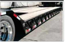
With a standard deck height of 22", Globe Trailers have lower overall height, which allows taller loads to be hauled.
