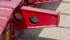
Globe Trailers fabricated heavy duty pullout front outriggers provide added strength which is needed to accommodate the initial force when loading equipment. The outrigger is held in position with a spring loaded locking pin.
