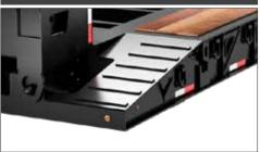
Low profile built-in integrated deck ramps.
