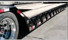
With a standard deck height of 22", Globe Trailers have lower overall height, which allows taller loads to be hauled.
