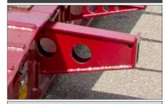
Globe Trailers fabricated heavy duty pullout front outriggers provide added strength which is needed to accommodate the initial force when loading equipment. The outrigger is held in position with a spring loaded locking pin.
