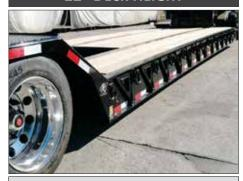
With a standard deck height of 22", Globe Trailers have lower overall height, which allows taller loads to be hauled.
