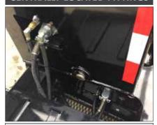
Air, electric and hydraulic (when applicable) fittings are all centrally located at the base of the gooseneck inside a bolster. This makes for quick and easy connect and disconnect.
