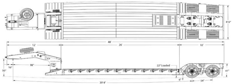
Trailer Model: GTBN352-48-26-GG Weight: Apx. \_\_\_\_\_\_ ± lbs
