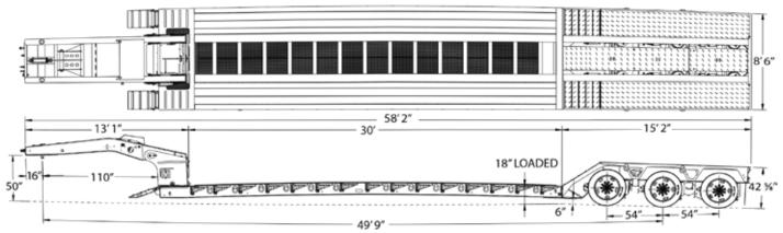
Trailer Model: GTBN503-57-30-HGG Weight: Apx.\_\_\_\_\_ ± lbs
