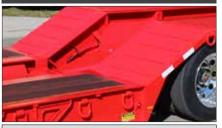
The 35 degree transition allows easier loading to the rear deck for equipment with lower ground clearance.
