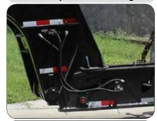
Air and Electric fittings are all centrally located at the base of the gooseneck. This makes for a quick and easy connect and disconnect.
