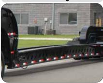
With a standard deck height of 24", Globe Trailers have lower overall height, which allows taller loads to be hauled.
