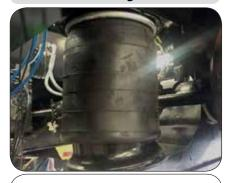
30,000 pound rated large diameter air bags are standard. This allows for lower operating pressure and higher capacity when needed.
