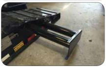
Heavy Duty, dual tubed steel pull out first outrigger.
