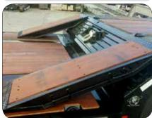
Adjustable sliding transition ramps with wood covering for traction. Ramps are removable.
