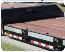
With a standard deck height of 20", Globe Trailers have lower overall height, which allows taller loads to be hauled.
