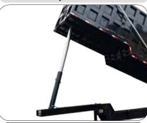
The hydraulic lift cylinder allows and restricts the trailer dumping angle up to 45°, which is optimal for ejecting debris and maintaining a safe operating height.
